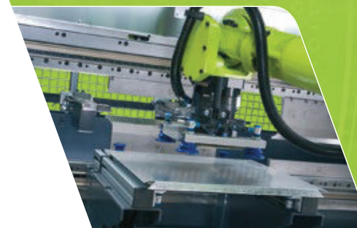
Turning over sheets
